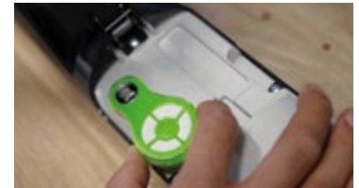
Possibility to unlock motor with transmitter
