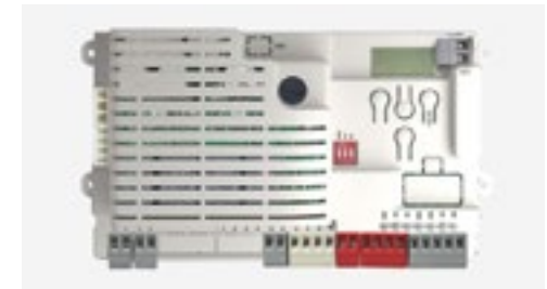
New control unit CTE20324 with integrated receiver programmable with KUBEPROW
